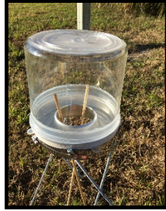
Fig. 2. Redesigned fire ant alate trap with dowel rods that guide alates into a collecting pan. Alates typically crawl to a high perch when they initiate mating flights.
